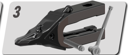
3 Insert helical pin and rotate 180 degrees with socket wrench to engage lock
